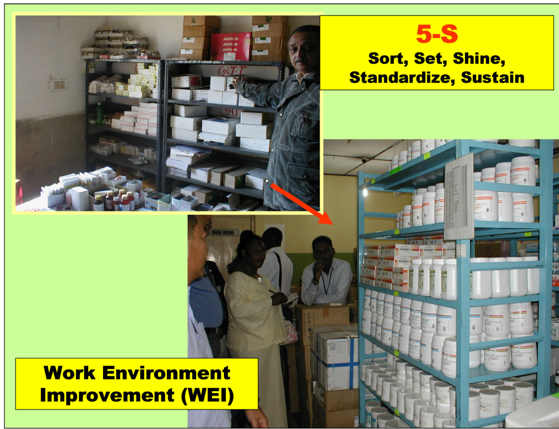
Figure 3-22: Before and after of 5S
